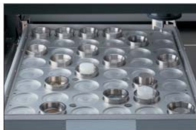
The sample changer with slide-out tray provides easy access to all sample positions utilizing the same sample holder for all sample types. The changer is upgradeable from 12 positions to 24, 36, or 48 positions.
